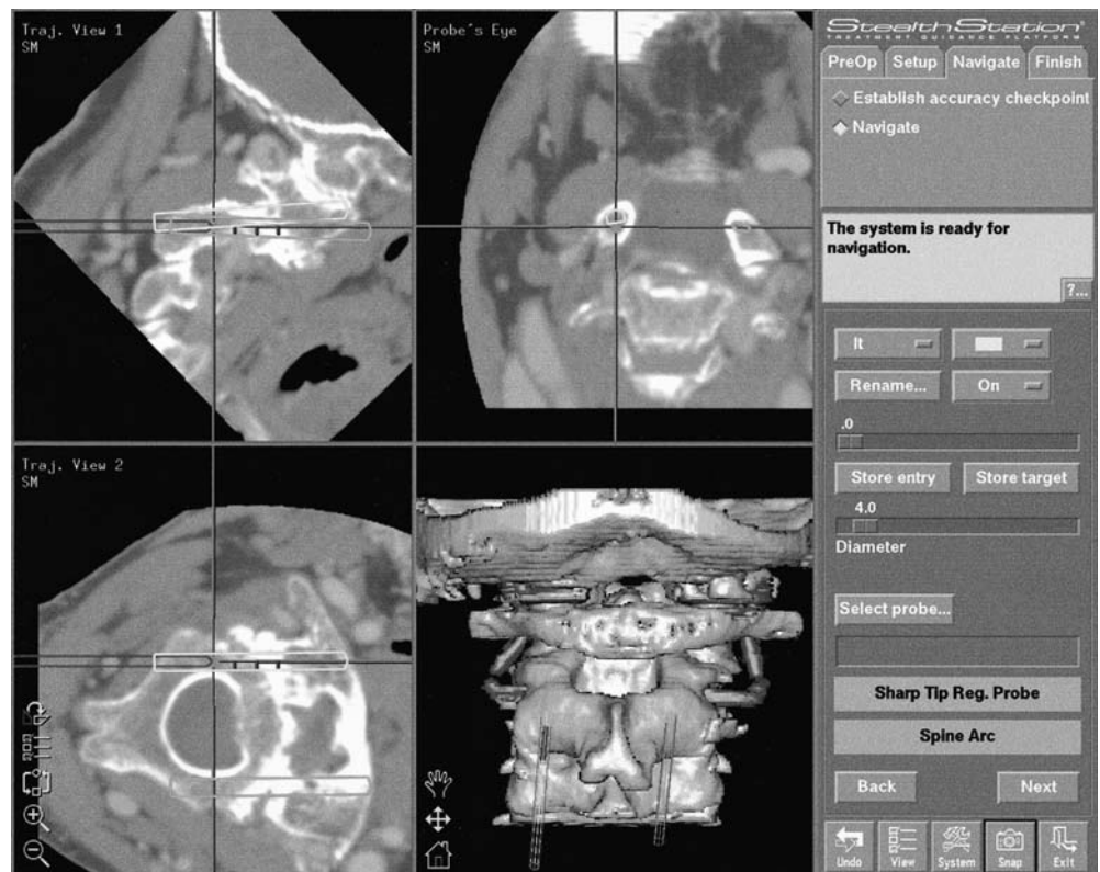
Fig. 2. Computer display shown at surgery. The position of the device and surgical plan are shown in four views. The wide white arrow indicates the position and direction of the device, and the narrow gray arrow indicates the planned screw trajectory
